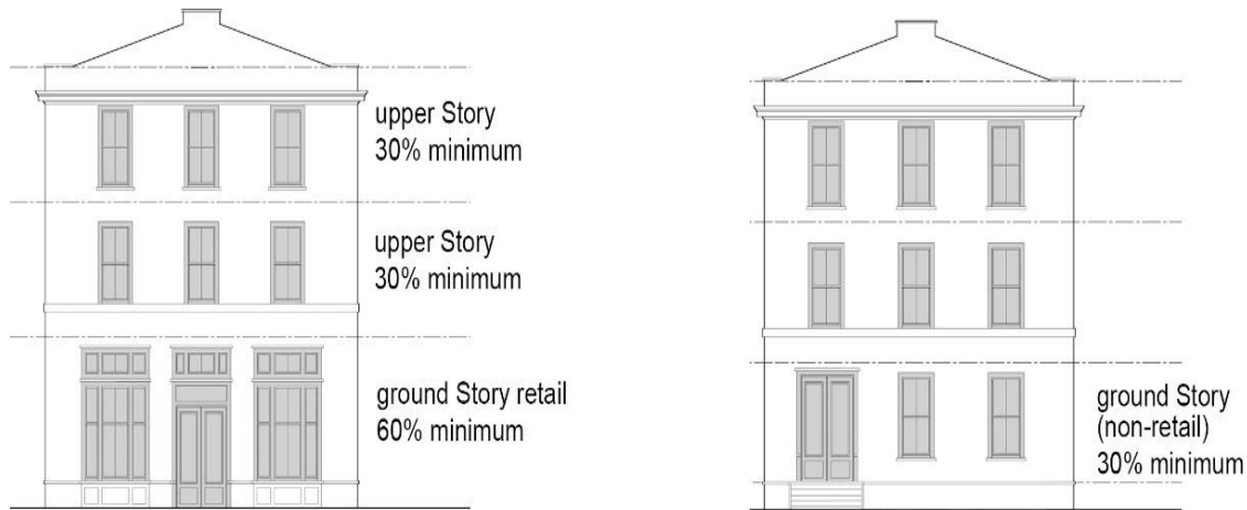
Figure 375-4-1: Minimum Façade Transparency Requirements
