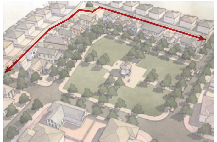
Rear Alleys Conceal Parking & Services
