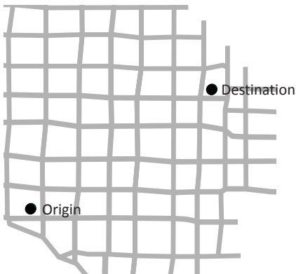
An 8x8 grid yields 12,870 possible routes from the origin to the destination
