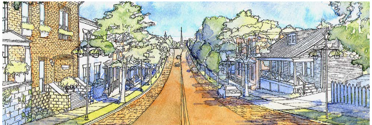
Scenario 2: By narrowing the lanes of Langhorne Road a second row of parallel parking can be added to the street. This additional row of cars functions as a traffic calming device as well as a buffer for pedestrians.
