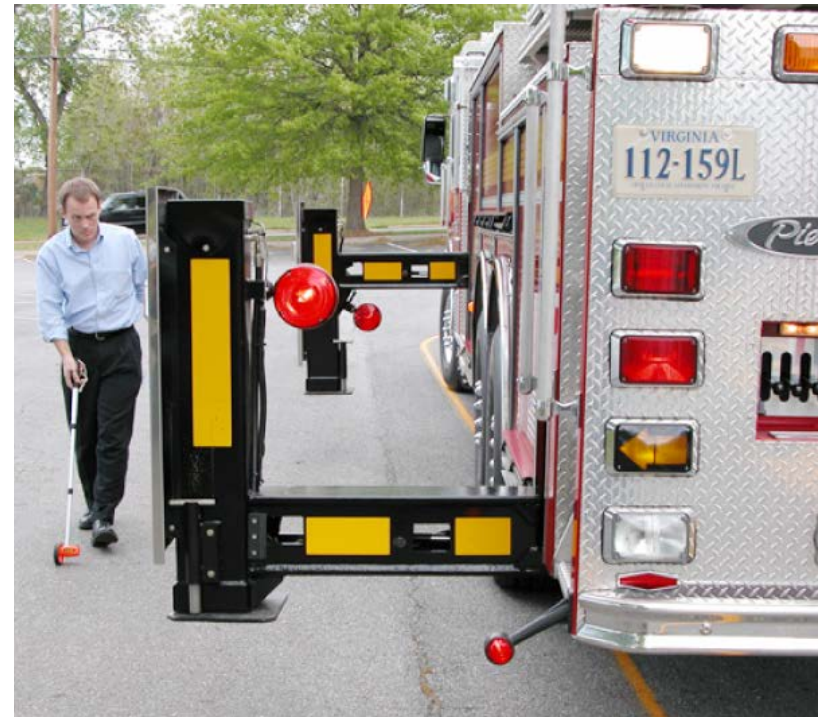
Figure 5: HPE staff measured Lynchburg Fire Department vehicles to create accurate turning specifications.
