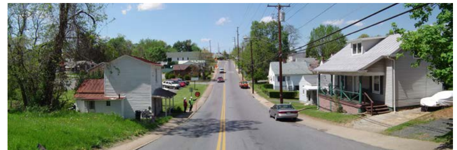
Scenario 2: By narrowing the lanes of Langhorne Road a second row of parallel parking can be added to the street. This additional row of cars functions as a traffic calming device as well as a buffer for pedestrians.
