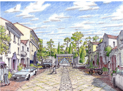
A plaza slopes toward a fountain and staircase. The plaza is detailed as a curbsless shared space, where parking, gathering area, and drainage features are distinguished by changes in paving materials and patterns.
