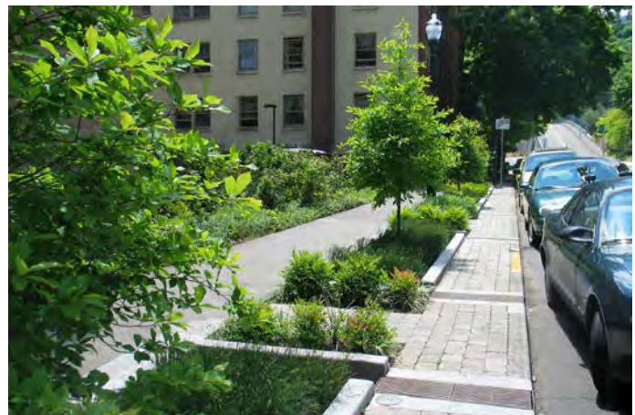
Tree wells can be used as a green infrastructure device to capture stormwater
