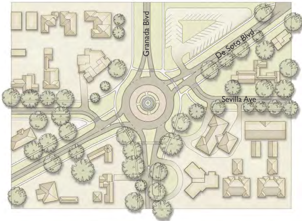
Option 3: Four-Point Roundabout - Merge De Soto Boulevard and Sevilla Avenue at both ends, resulting in more curb changes and fewer splitter islands.
