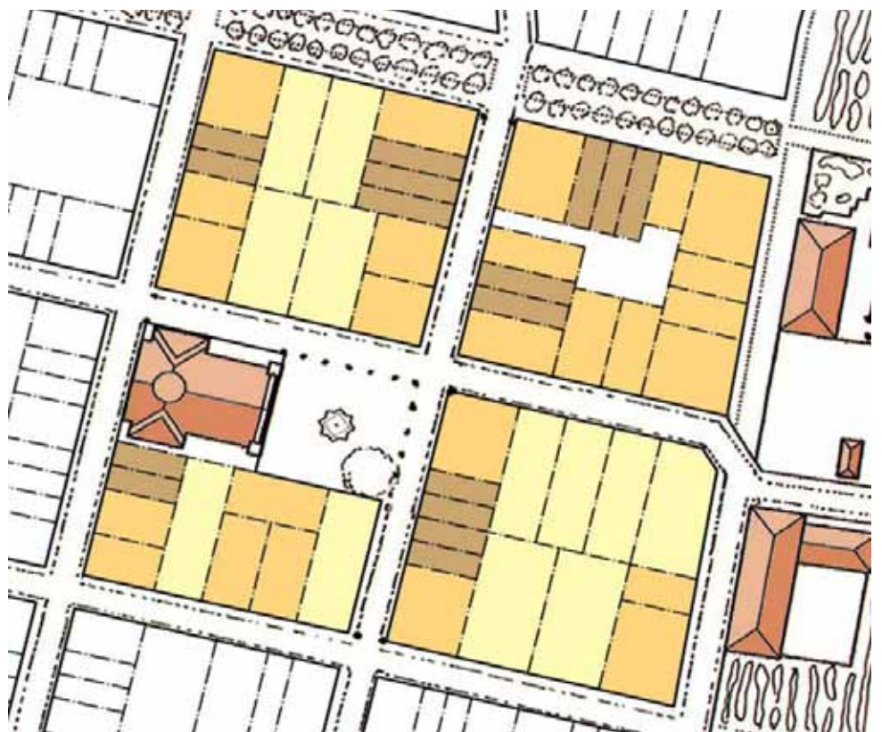
Courtyard types are arranged in different configurations to form blocks.
